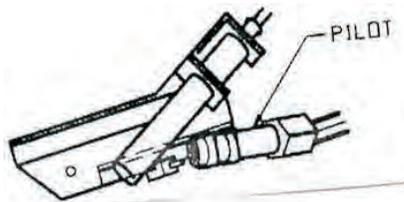
8. Once the pilot remains lit, depress the gas control knob slightly and turn the gas control knob counterclockwise ↶ to "ON." NOTE: The "ON/OFF" SWITCH is used to turn the flame on or off when the control valve is in the "ON" position.
