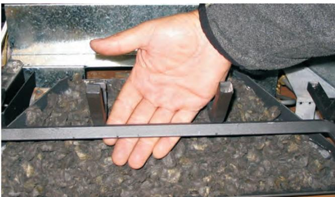
Step 4: Once the wool is in place, check the gap between the grate bar and the wool. It should be about the thickness of your hand. (Approximately 3/4")\_
