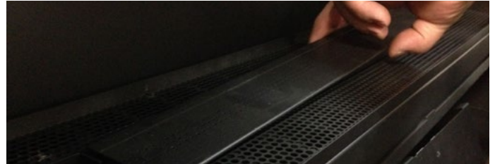
Figure 13.b Loosening the venturi
