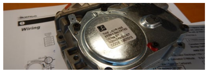
Figure 13.k Conversion label on valve
