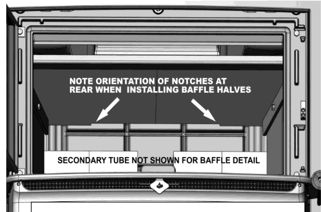
Figure 11 - Baffle Notch Detail
